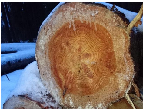
Figure 1. Heartwood and sapwood are visibly different in Scots pine.
