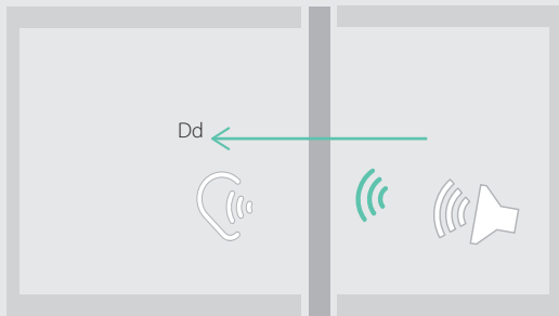
Figure 1.4 Laboratory measurement of the sound reduction index R: direct transmission path.
