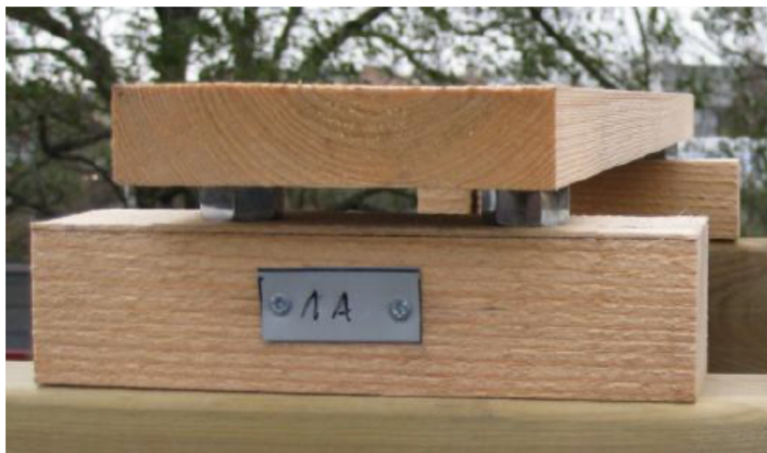
Figure 2.4. Reference element for climate exposure – horizontally exposed spruce board without moisture traps. (Photo: Tord Isaksson, Lund University).
