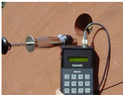
Figure 6.8. Moisture meter with slide hammer
