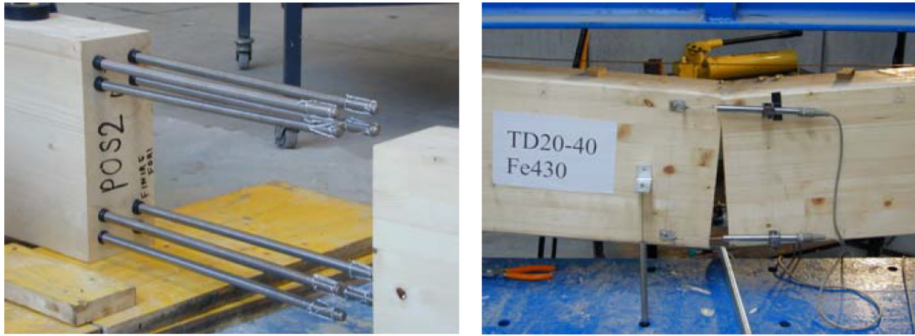
Figure 3.55 Splice joint with glued-in rods, left: rods glued into one member of the joint, right: deformation of the joint, (Gattesco, Gubana et al. 2010)
