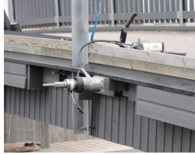
Figure 6.11. Load cell measuring tension force in bars
