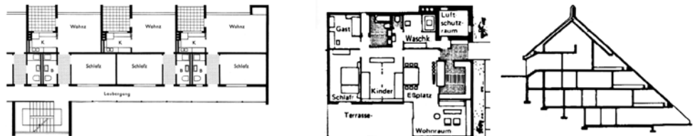
15. Typological floor plans with centralised access (from left t. r.): double dwelling, triple dwelling, staggered dwelling, Point block, acc. t. Neufert, 1973.
