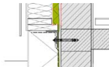
161. Brackets and sill beam as linear anchoring solution with decoupling on the sill..
