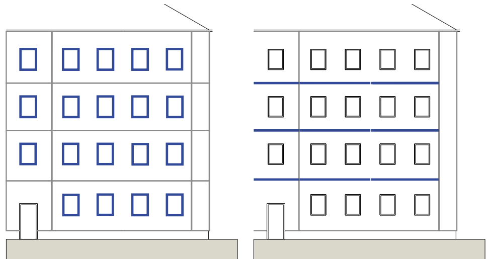
147. Partitioning with fire stops in order to prevent the spread of fire a) fire stops around windows b) horizontally storey-wise separation of the elements.
