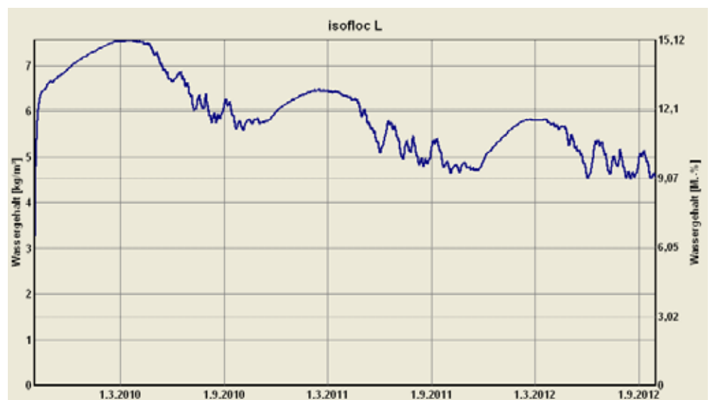
159. Humidity diagram of the cellulose fibre insulation layer shows the good drying capabilities during a range of three years. The overall mass of moisture in the element decreases.
