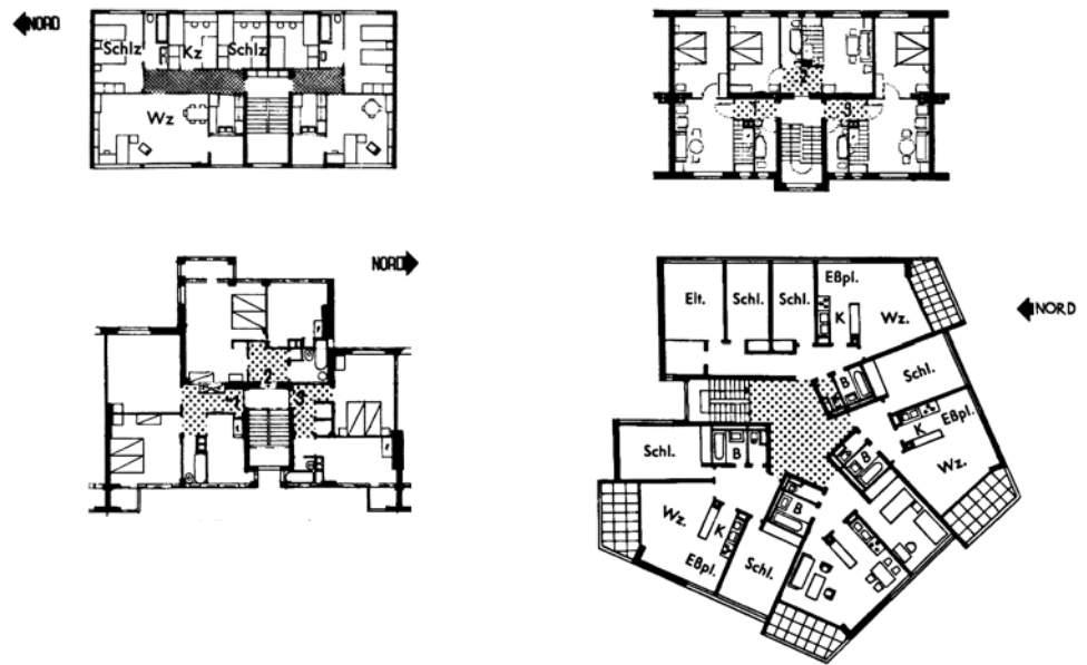
14. Typological floor plans with corridor houses and terraced houses (from left t. r.): acc. to Neufert, 1973.
