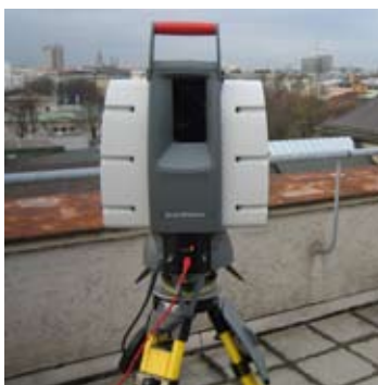
70. Full featured 360° 3D Laser-scanner on a tripod.
