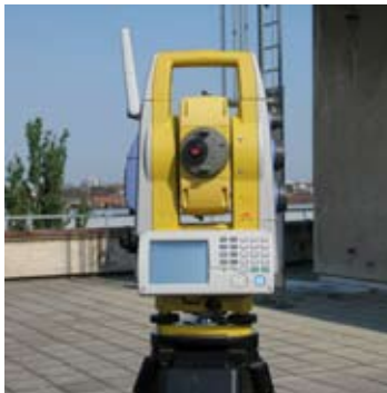
69. A modern Tacheometer also called Totalstation.
