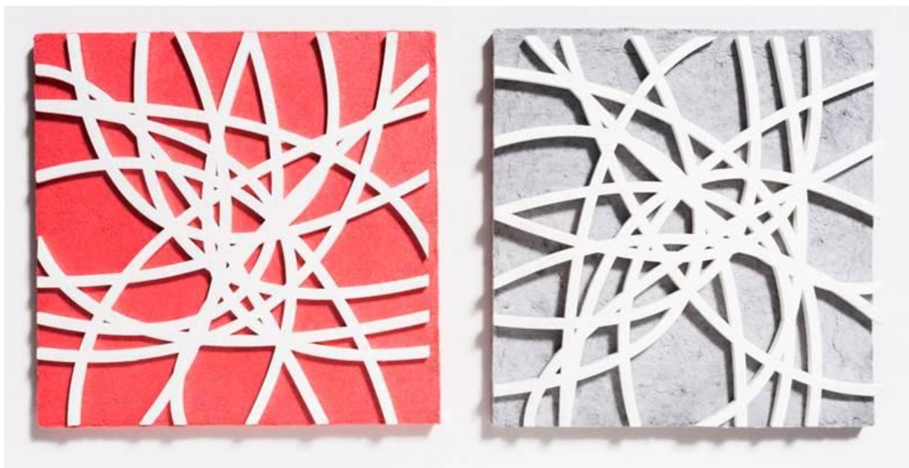
Figure. Two layered demo panels (40cm x 40 cm) for décor and sound absorbance purposes by Jani Lehmonen, VTT (material and process) and by Heidi Turunen, Aalto university (design). Base material is pure pulp. The panels are produced by foam forming and pressed to desired density profile. In the bottom panel the pulp was dyed before foam forming. The top panel (white) is water cut to beautiful shapes. Photo by Eeva Suorlahti.
