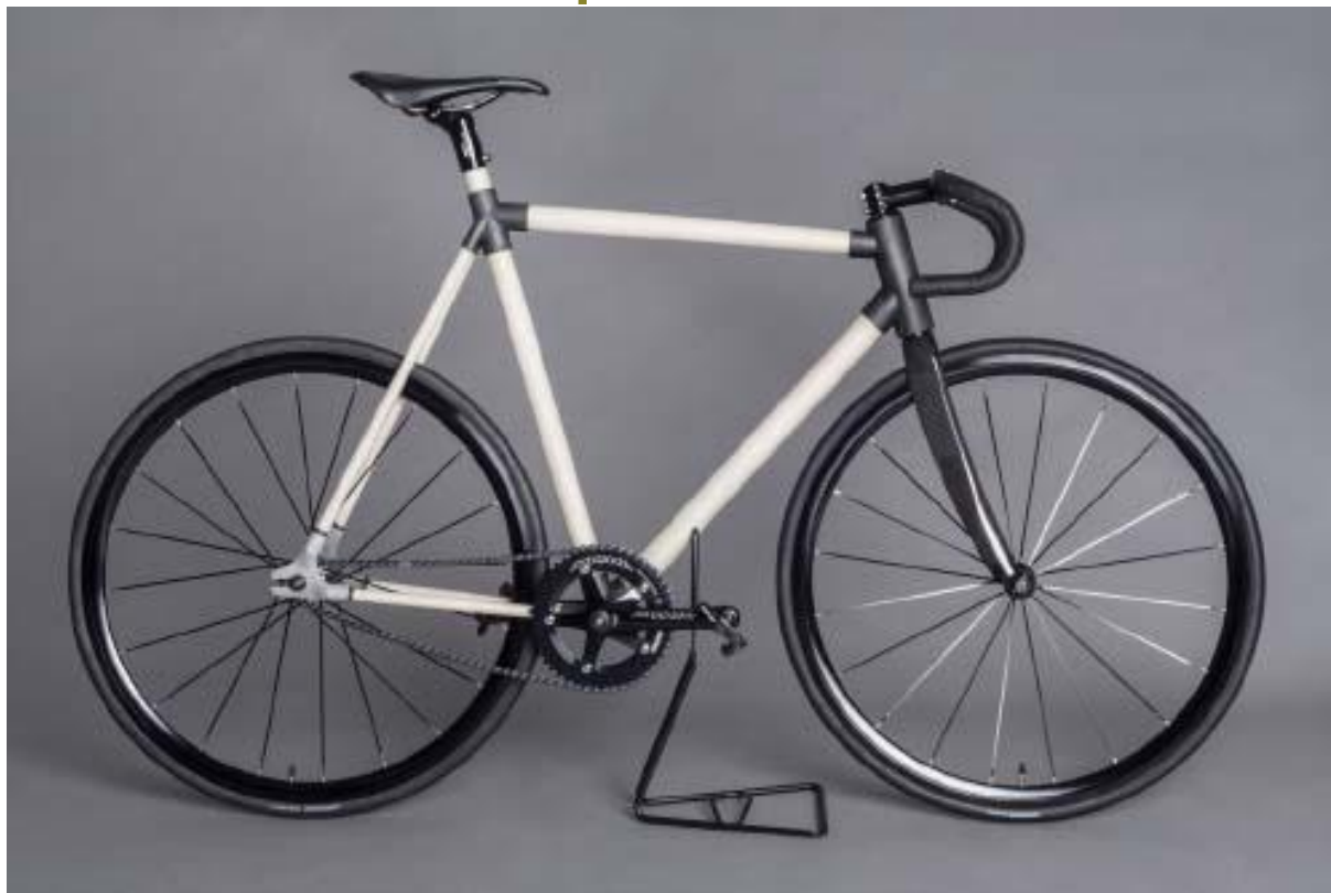
Figure. Concept bike with load-bearing nanocellulose tubes (white structures). Bike was produced by Tiina Härkäsalmi and Kim Antin /Aalto, and Tuomas Pärnänen TUT. Testing of the mechanical strength of the CNF tubes has been done by Mauno Kemppainen and Steve Spoljaric (Aalto). Photo by Eeva Suorlahti.
