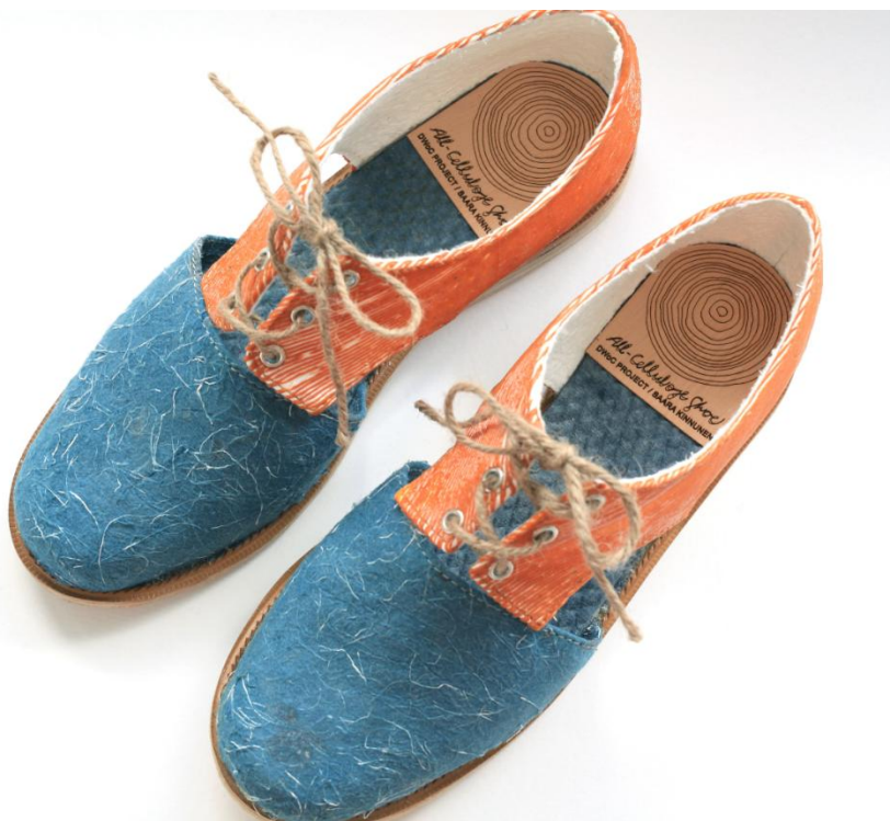
Figure. Shoe demonstration. Upper material is strong, cellulose based nonwoven textile. The brown texture is made by 3D printing cellulosic paste on cellulose non-woven. Saara Kinnunen HAMK, Jukka Ketoja, Atsushi Tanaka and Kirsi Kataja, VTT. Photo by Saara Kinnunen.
