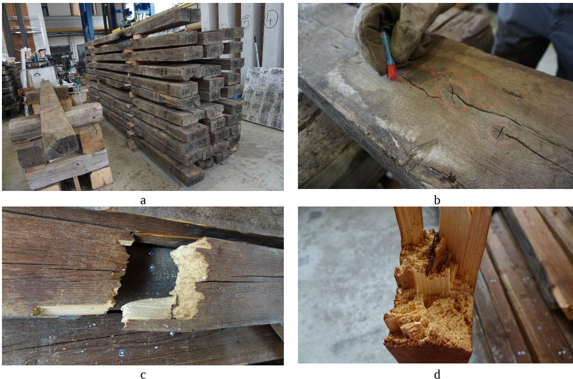
Figure 5.4 a) old oak b) investigation of properties c)-d) Recovered wood with brittle failure
