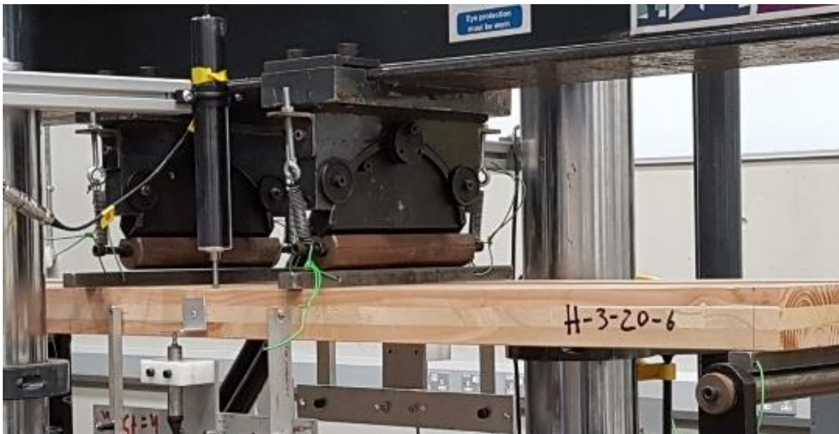
Figure 3.3 Test of CLT from reused timber.
