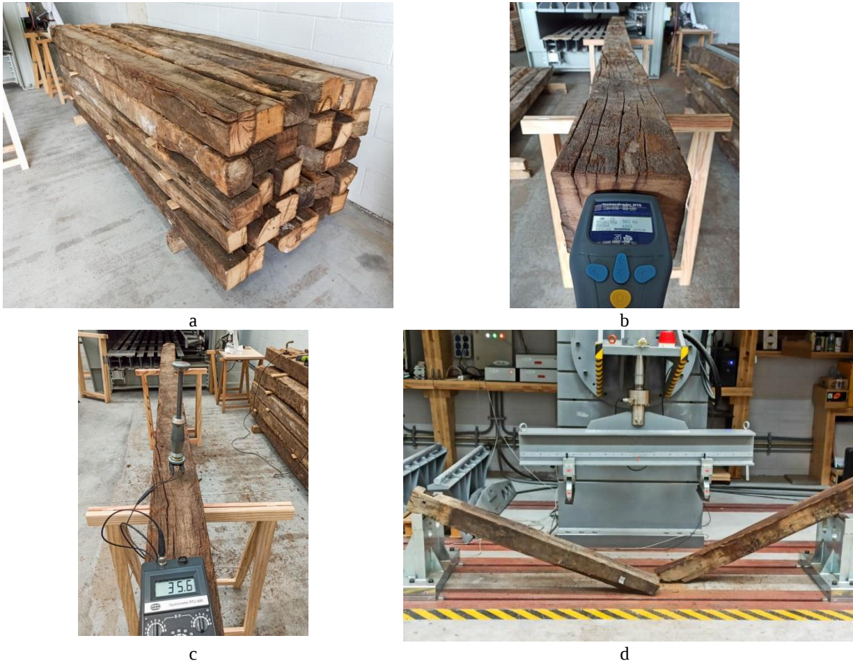
Figure 5.7 a) Spanish recovered oak b) non-destructive testing c) moisture content estimation d) four-point bending test.
